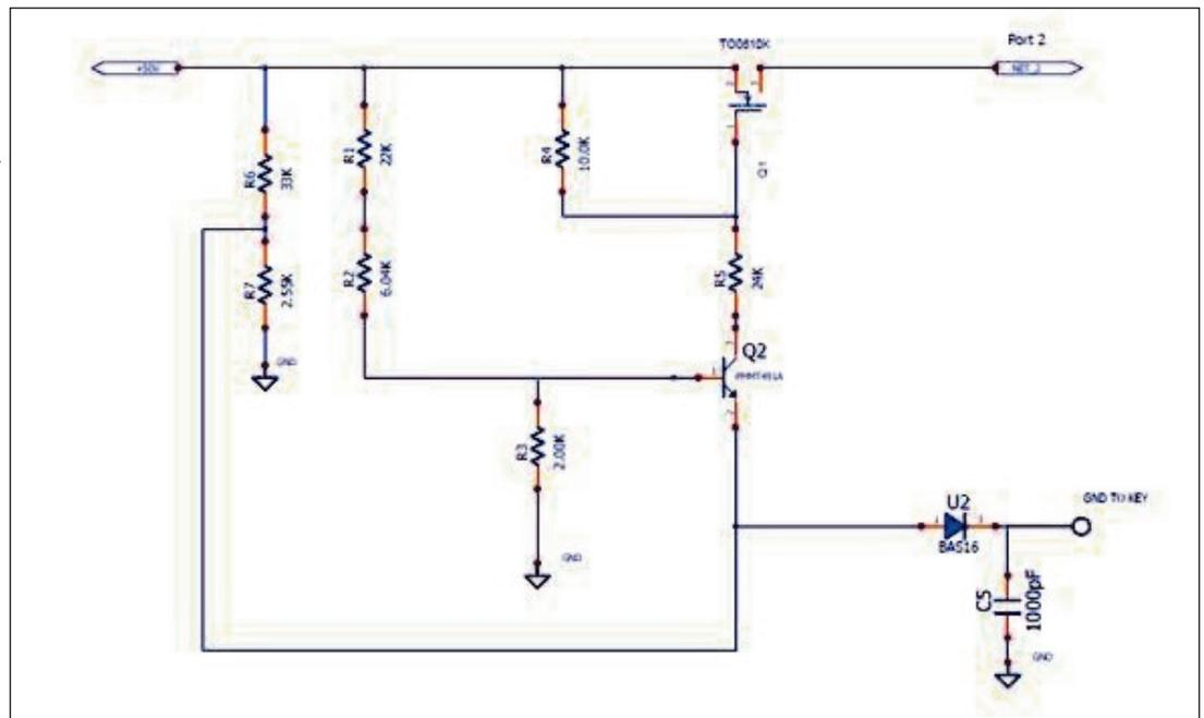
This works well. The Larcan bias current is about 12 mA, and the voltage on the key line is only 2.2V using a 50V supply. The theory of operation is the same as the original design. The FET gate is held high with R4, and the transistor (Q2) is not conducting in receive. Grounding the PTT line, causes Q2 to conduct, lowering the gate voltage to the drop across R5 and the FET now conducts. The P channel FET chosen had a current rating of 150mA.
