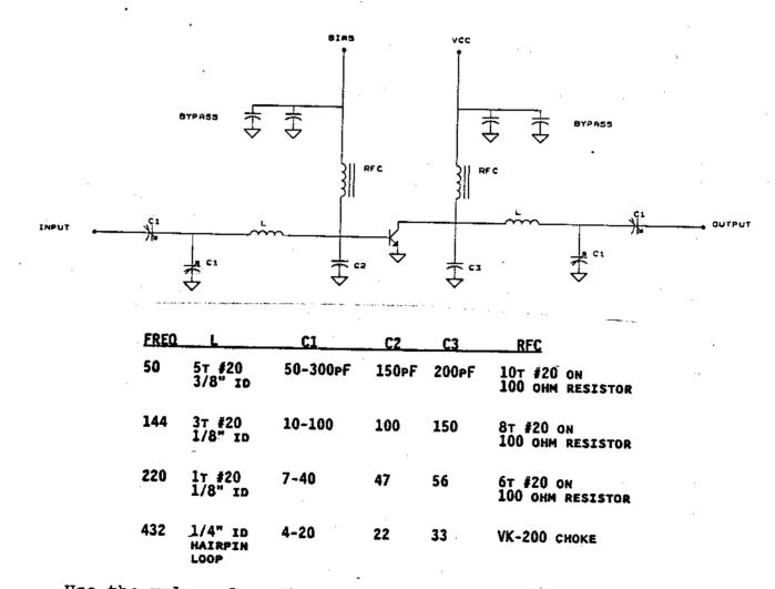
Use the values from the table as a starting point. Use your favorite bias circuit, apply RF and tune the input match for lowest input VSWR and then the output for maximum power. WB3JYO 9-89
