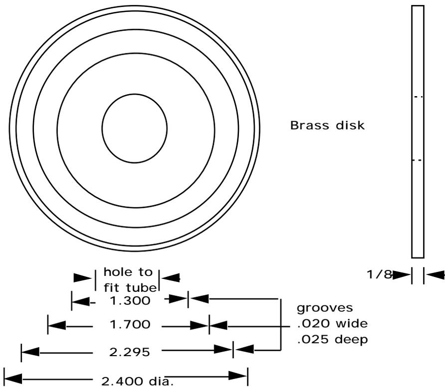
Turn the 2 1/2 dia. by 1/8 thick disk to 2.400 in dia. and drill and bore the center hole to a size that allows you to push the tube thru with some effort. Machine the grooves to dimensions shown (this is the tricky part).
