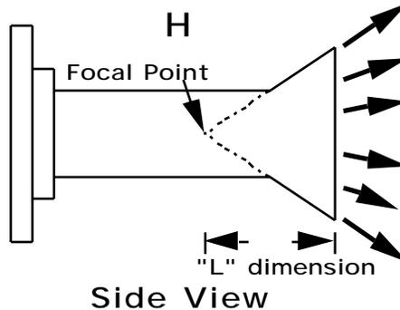
NOTE: This feed should be mounted on the dish so that the focal point of the feed is at the focal point of the Dish
