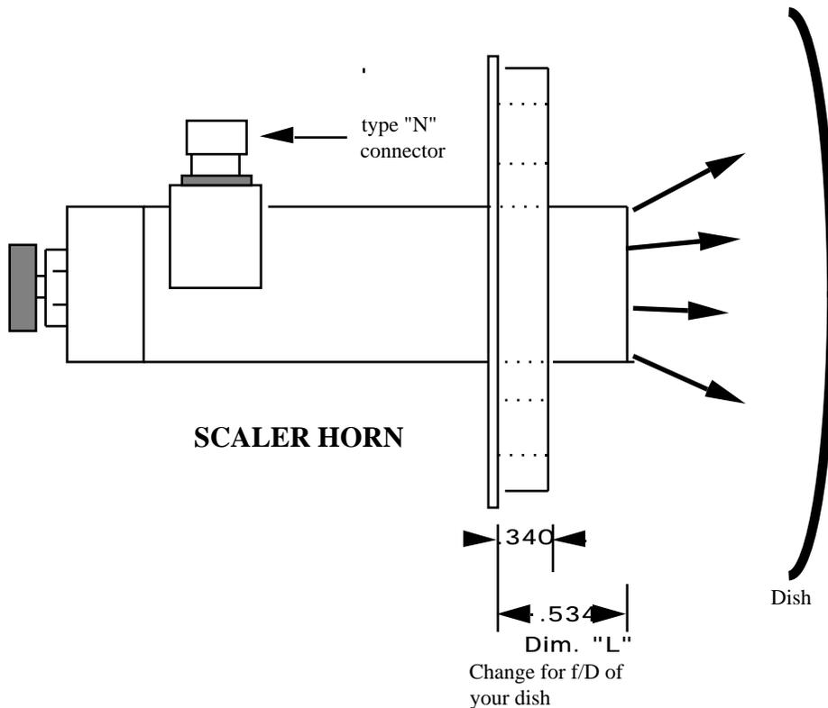
This feed was designed for a reflector with a f/D of .375, The "L" dimension determines the beamwidth of the feed, if you have a dish with a different f/D "L" will have to change.
