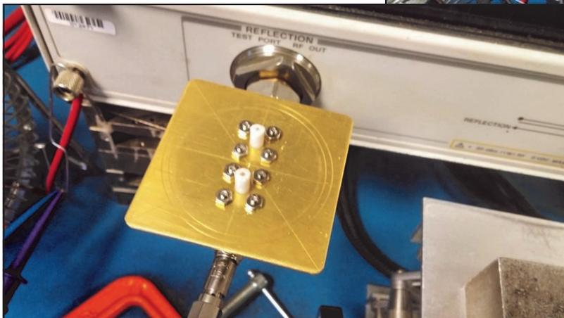
As you can see, Doug includes real craftsmanship in his builds. The SMA connectors are the kind with Teflon sleeves (used to pass through machined housings). I wonder if the exposed nuts have any effect on the filter characteristics?
