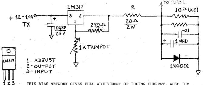
THIS BIAS NETWORK GIVES FULL ADJUSTMENT OF IDLING CURRENT. ALSO THE DROPPING RESISTOR CAN BE A LOT SMALLER IN WATTAGE. THIS MAY BE USED FOR ANY AMPLIFIER. WASJUF
