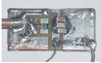
Offset of double sided PCB 1.6mm (Run wires through PCB near the resistors and capacitors)
