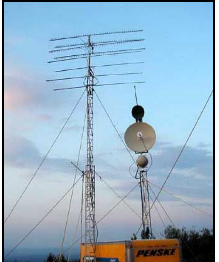
1296 & 903 arrays 2-3-5G dish between 10G & 24G dishes
