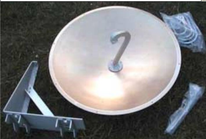
I unpacked this new from the box. This was made by MA/COM for their RAPAC system and consists of a two foot dish antenna with a button hook feed, pole mount, brackets, clamps and all hardware. This dish has about 33 dB of gain, the button hook terminates in WR-90 four hole flange waveguide, has a Kapton weather window and is beautifully made. This dish is very sturdy and will not warp or twist in the wind. Kmec@aol.com
